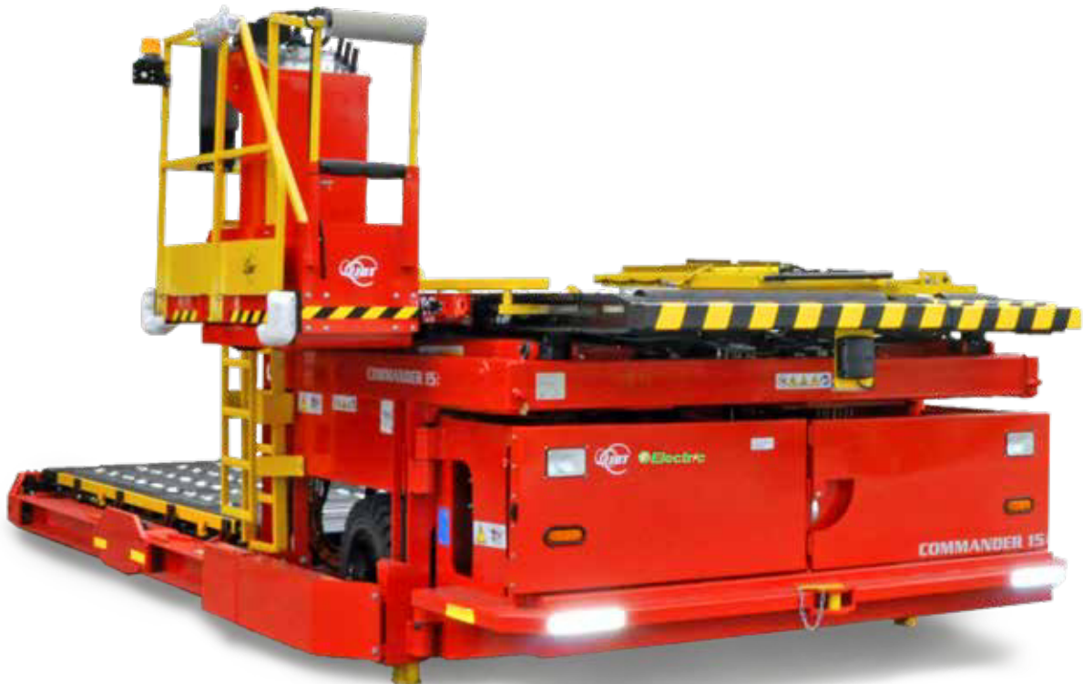
A JBT C15i loader with ASO's SENTIR safety contact bumper
